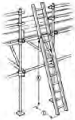
Figure 13.11 Correct Ladder Angle
